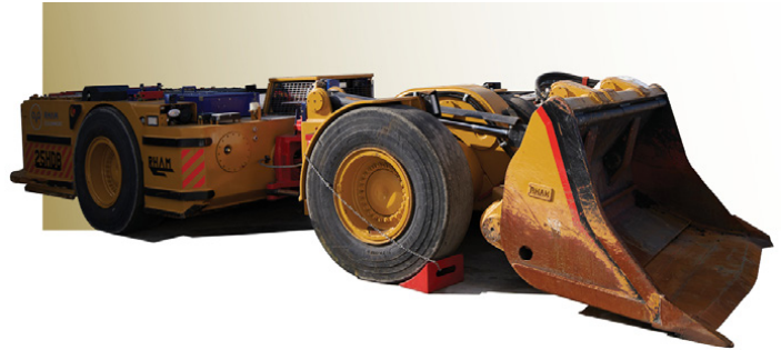
Remotely operated battery-electric LHD at the Bathopele operation at SA PGM
