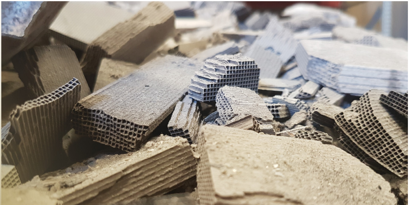
Spent autocatalysts are recycled at the US PGMs Columbus metallurgical complex to output PGMs
