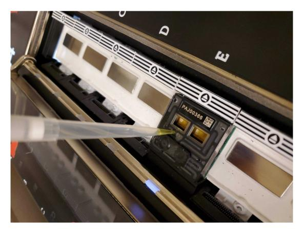
Flush 500ul of the priming mix into the inlet port and close the port. Wait for 15 mins.
