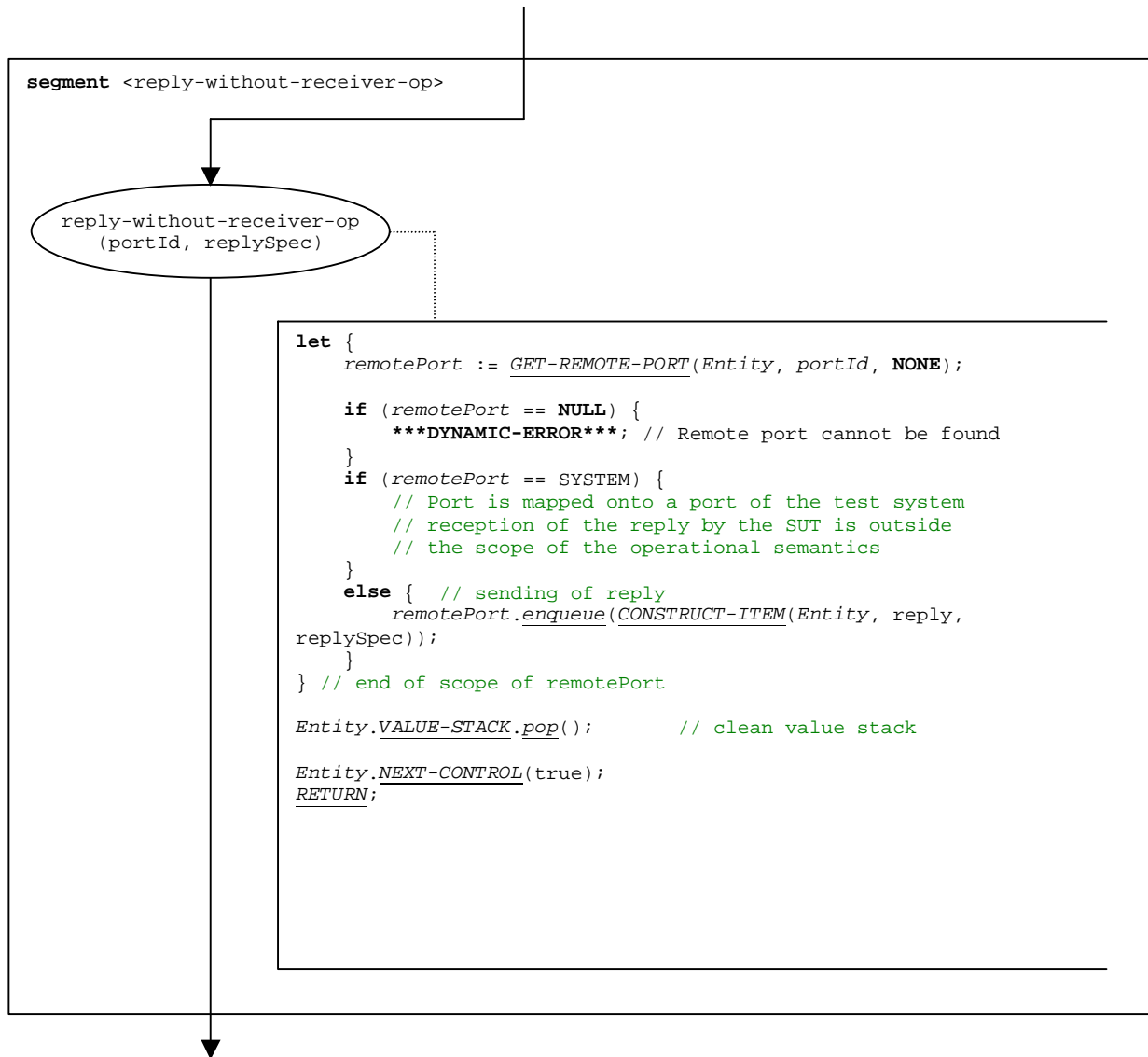
Figure B.98: Flow graph segment <reply-without-receiver-op>
