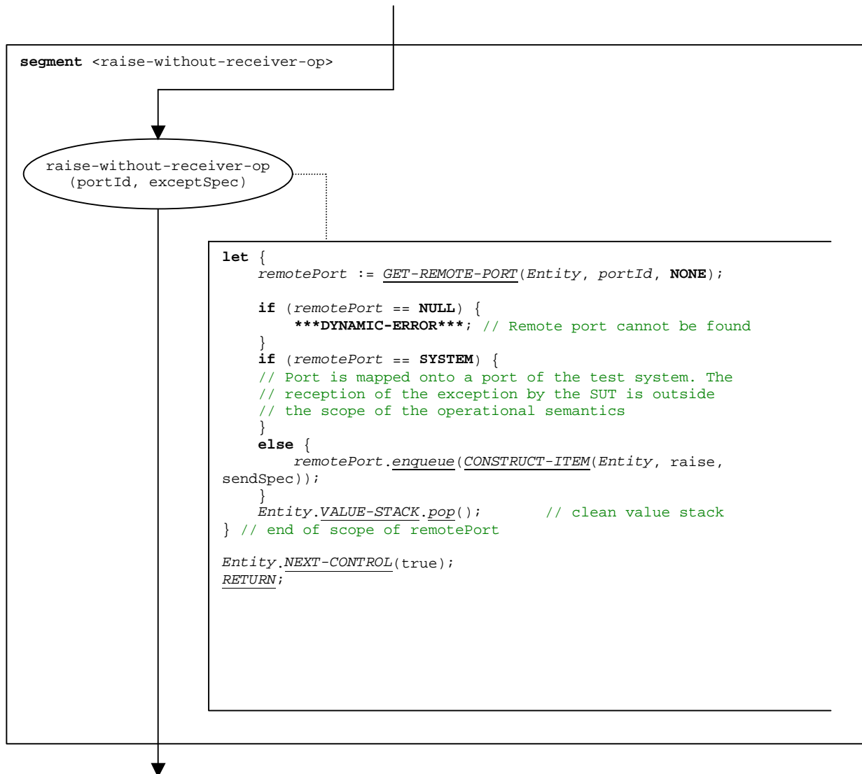
Figure B.90: Flow graph segment <raise-without-receiver-op>
