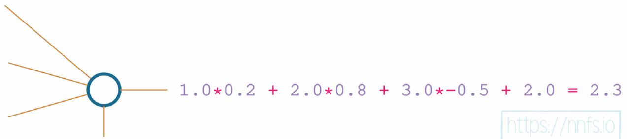
Fig 2.01: Visualizing the code that makes up the math of a basic neuron.
