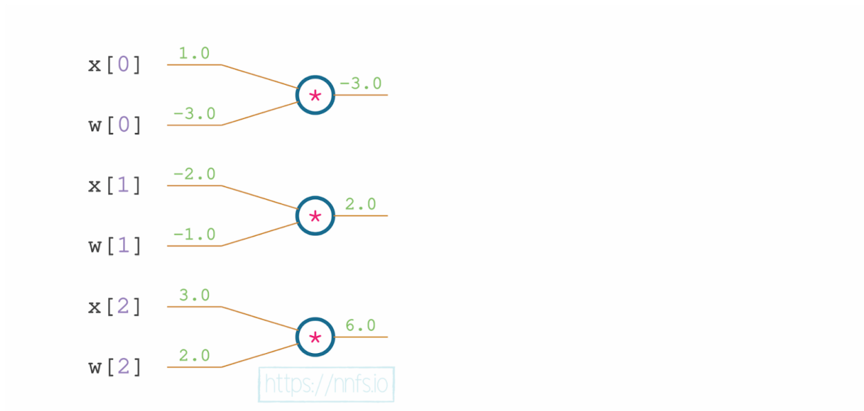
Fig 9.03: Input and weight multiplication of all of the inputs.
