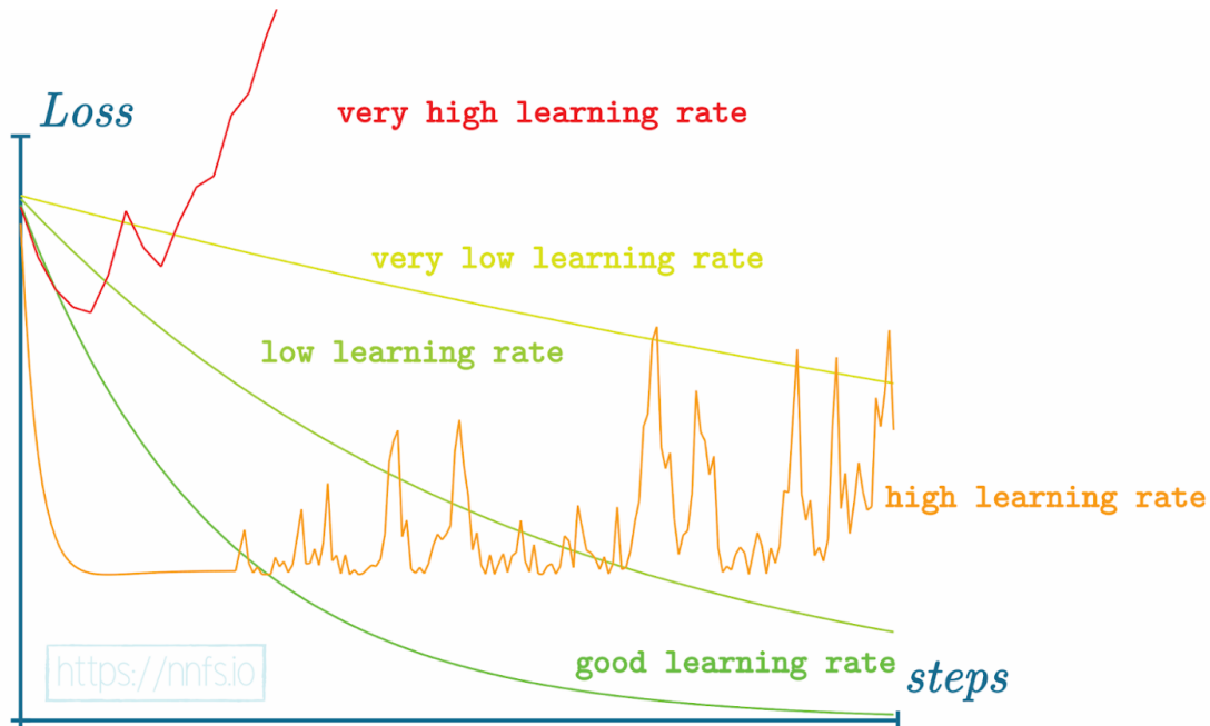
Fig 10.14: Graphs of the loss in a function of steps, different rates
