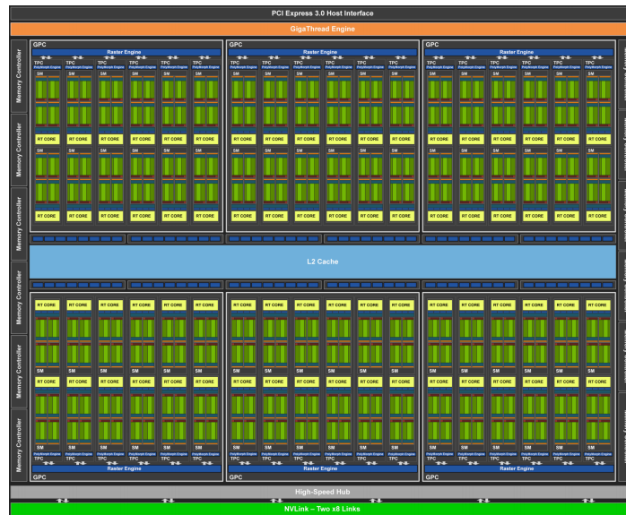
Fig. 12.4.8: NVIDIA Turing architecture (image courtesy of NVIDIA)
