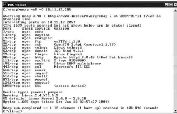
Figure 11-5: Using Nmap to determine the OS kernel version of a Linux server.
