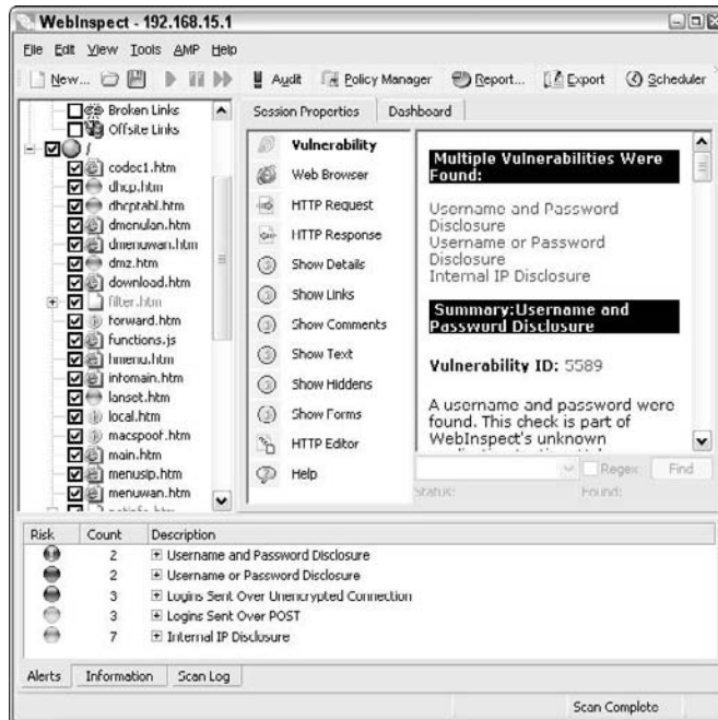
Figure 13-14: Websinspect scan of a VoIP network adapter showing several weaknesses.
