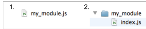
Figure 3.3 Node modules can be created by using either files (example 1) or directories (example 2).
