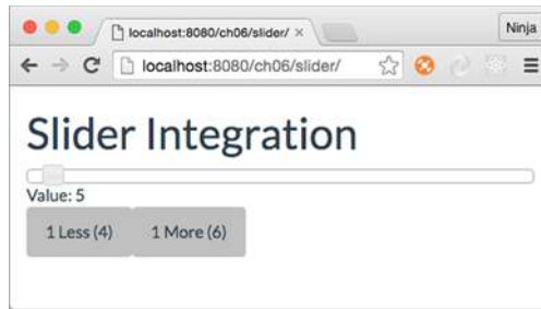
Figure 6.14 React components (buttons and the text “Value: …”) can be integrated with other libraries, such as jQuery Slider, to make all elements from all libraries communicate with each other.
